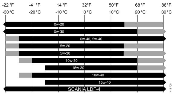
The illustration describes which ambient temperature in °C the viscosity class can handle for Scania-approved and market-approved oil grades. Note that the Scania-approved oil grades have a greater temperature range than market approved oil grades.
