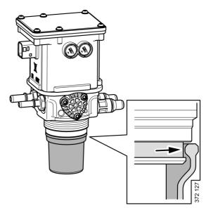
7. Lubricate the sealing diaphragm and threads with the accompanying spray.
