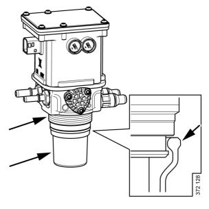
8. Renew the O-ring. Place the new O-ring in the filter housing.
