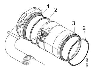
16. Fit the V-clamp (2) and the band clamp (1) loosely around the particulate filter.
