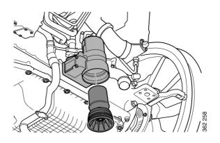
10. Remove the rotor by pulling it straight up from the cover. See illustration.
