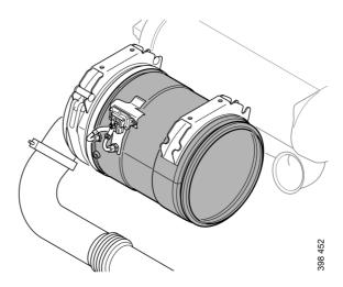
8. Detach the differential pressure sensor connections and remove the nut from the bracket.
