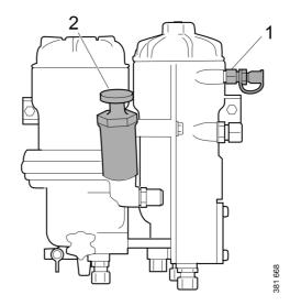
Engines with a bleed nipple in the fuel filter housing
