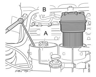
8. Move the suction tool to the main filter housing (B). Draw out remaining fuel and particles.
