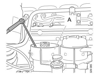
5. Make a mark on the main filter cover (B). Unscrew the cover 3 to 4 turns with the socket. Draw out fuel which may drain into the water separating prefilter housing when the main filter is detached.
