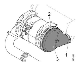
6. Remove the V-clamp (2) and the band clamp around the particulate filter (1).
