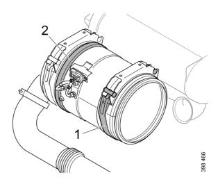
17. Align the particulate filter outlet for the differential pressure sensor with the mark. Tighten the V-clamp and the band clamp around the particulate filter. Tightening torque, V-clamp, 20 Nm.
