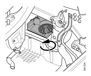
9. Remove the bottom cover together with the rotor.
