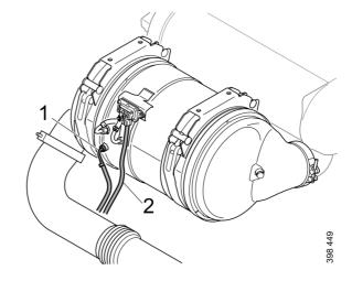
3. To facilitate fitting, use a marker pen to mark the position of the particulate filter. Make a mark on the oxidation catalytic converter in line with the particulate filter connections for the differential pressure sensor.
