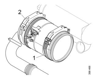
7. Lift off the particulate filter carefully.
